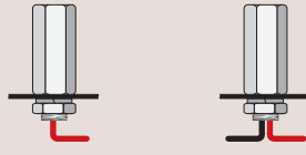
FS7008 Easy Mount Adapter with 6" Hot Wire Pigtail FS7008-2 Easy Mount Adapter with 6" Hot Wire and Ground Wire Pigtails
